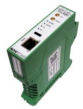
The FLL400 functions as a repeater, extending the transmission range and enhancing the reliability of data being broadcast in challenging environments.
